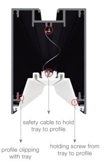
System with front removable tray which permits easy access to the led strip and power supply, therefore allowing very fast and simple maintenance.
