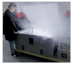
Salt spray chamber (corrosion tester):
