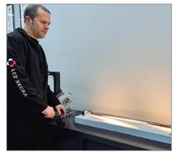
Torsion testing for flexible led strips:
